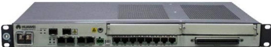
Figure 6. MA5612 DC; 10G PON upstream transmission:
