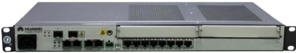
Figure 4. MA5612 DC; without POTS port:
