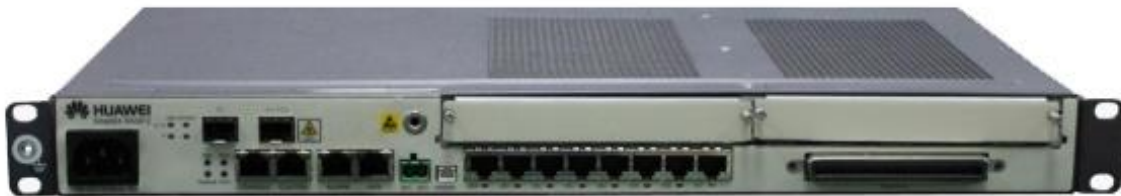
Figure 6. MA5612 DC; 10G PON upstream transmission:
