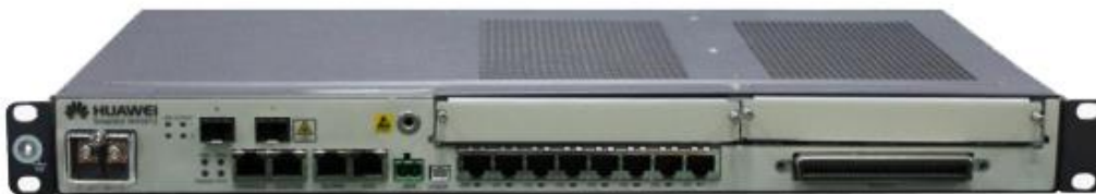
Figure 3. MA5612 AC; without POTS port:
