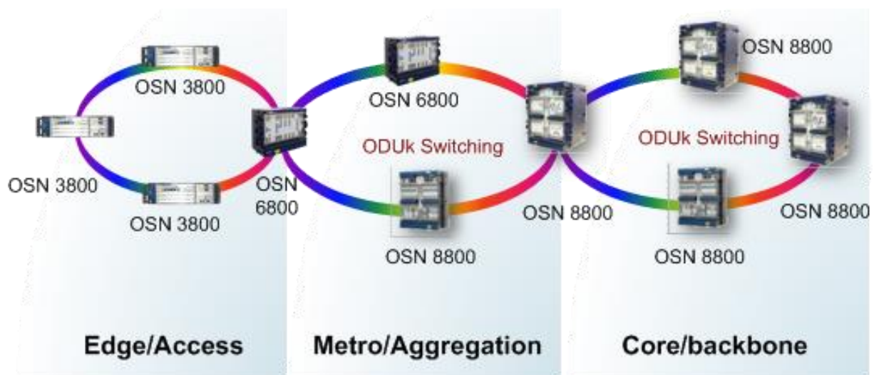
Position of the OptiX OSN 3800 / 6800 in the network hierarchy
