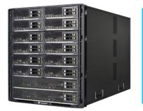
The E9000 chassis is engineered as a 12U 16-blade form factor. It provides a fully redundant modular design for power supply, heat dissipation, management, and switching.
