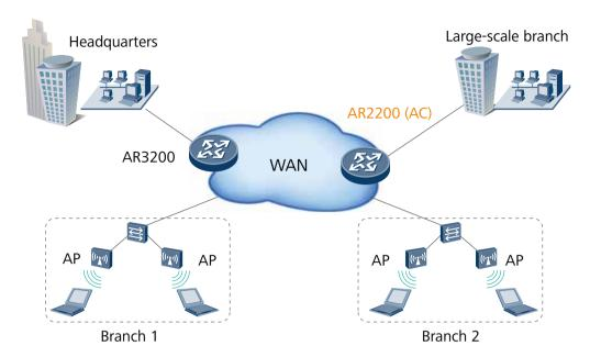
The AR2200 routers integrate AC (Access Controller) functionality, which can manage the wireless AP (Access Point) in wireless LAN. AR2200 supports rich certification and flexible user access control, which can provide security access quarantee for Wi-Fi users. The rich wireless capabilities integrated in one device, this can realize centralized management of wired and wireless networks, to meet the requirements of different scale enterprises networks.
