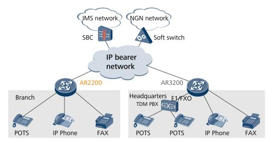
The AR2200 integrates voice, fax, and IP services. For enterprise users, the AR2200 serves as the SIP access gateway for a branch office, transforming phone signals into VoIP signals. The AR2200 uplink interfaces connect to the IP Multimedia Subsystem (IMS) or Next Generation Network (NGN) to allow any media, including phones, handsets, and computers to communicate at any time.
