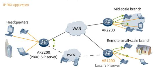
To enhance the corporate image and improve communication efficiency, all AR routers include a built-in PBX. This feature supports the enterprise main number, Interactive Voice Response (IVR), and bill query functions. The AR1200 can also be located in a branch office to provide intelligent dialing.
