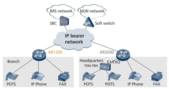
The AR1200 integrates voice, fax, and IP services. For enterprise users, the AR1200 serves as the SIP access gateway for a branch office, transforming phone signals into VoIP signals. The AR1200 uplink interfaces connect to the IP Multimedia Subsystem (IMS) or Next Generation Network (NGN) to allow any media, including phones, handsets, and computers, to communicate at any time.
