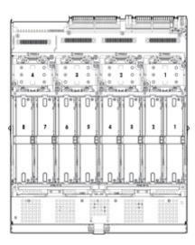
The server can operate in independent channel mode (performance) or combined channel mode (lockstep). Lockstep mode improves the system reliability and availability. If running with RDIMM (built with x4 DRAM devices), the system can survive the complete failure of two DRAM devices (DDDC). Running in independent mode, the server can only survive the complete failure of a single DRAM device (SDDC).
